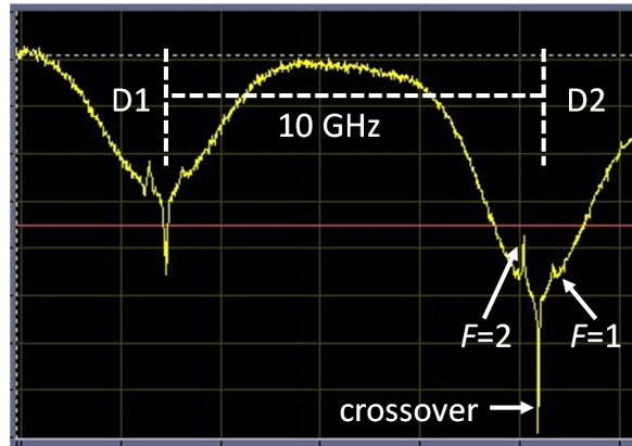
Figure 3.2: Example scan of the master laser across the D1 and D2 transitions showing the hyperfine sublevels. The master laser is locked to the crossover resonance between the F = 1 and F = 2 ground states.
