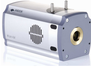
Figure 5.8: An iKon-M Andor camera was used to detect bremsstrahlung photons produced by the LWFA electron beam. The quantum efficiency of the camera is shown on the right, where the dashed green line (BN) corresponds to the camera used for this setup.
