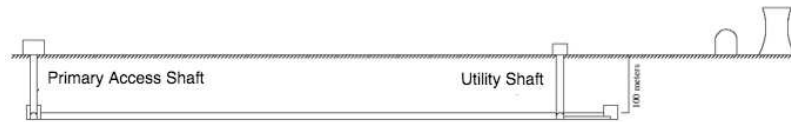
Figure 4. Proposal for an underground neutrino laboratory at the Braidwood nuclear power plant in Illinois using vertical access shafts.
