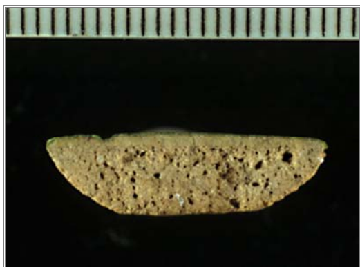
Figure 1. Cross section through a faience inlay from Tell el-Amarna. The upper surface, a thin layer of greenish glaze, tops a layer of very fine faience and a coarse layer beneath. This piece was probably glazed by efflorescence.
