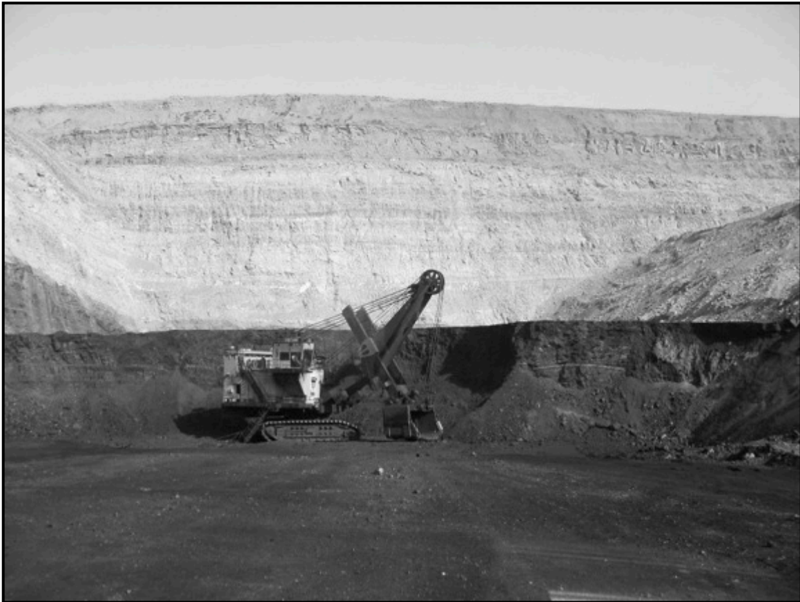
Figure 7. A view from the pit base in the Heidaigou coalmine in Xuejiawan Township, Jungar Banner, Ordos Municipality, 2011. The coal seam is visible as the black portion beneath approximately 20m of rock.
