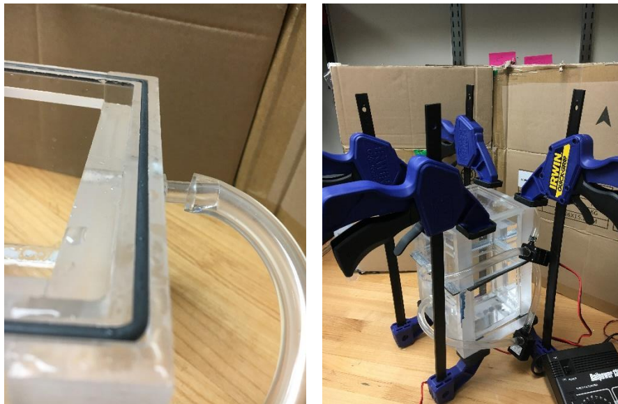
Figure F3. a) Gasket running around the top edge of the lower chamber. b) Clamping added to maintain seal between chambers.
