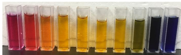
Figure 3.4. Thymol blue pH indicator at pH values of 1 to 10 in steps of 1 (from left to right).
