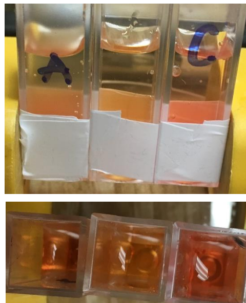
Figure 3.5. Digital photographs of the ED cell after 9 V was applied across the cell for 30 min and thymol blue pH indicator was added: (top) front view (bottom) top-down view. Originally, each of these three chambers contained 5 mM \text{H}_2\text{SO}_4 and was completely colorless.
