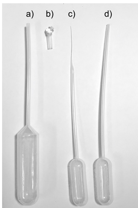
Figure 2-5 Pipettes used for titration, including a) A 15.3 mL pipette with b) Tygon®-tubing cap, c) modified tip of a d) 4.5 mL pipette.
