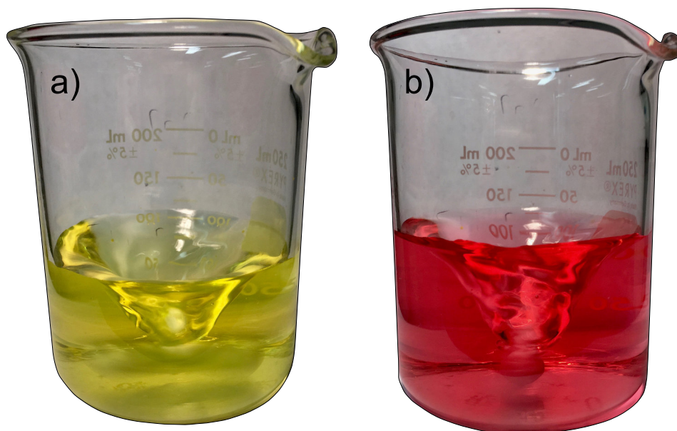
Figure 2-6 Color of sample after a) addition of indicator and after b) reaching the titration endpoint.
