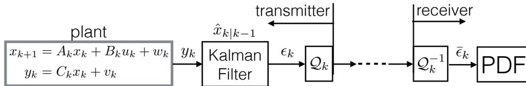
**Figure 5.1.** Block diagram of quantized innovations system.
