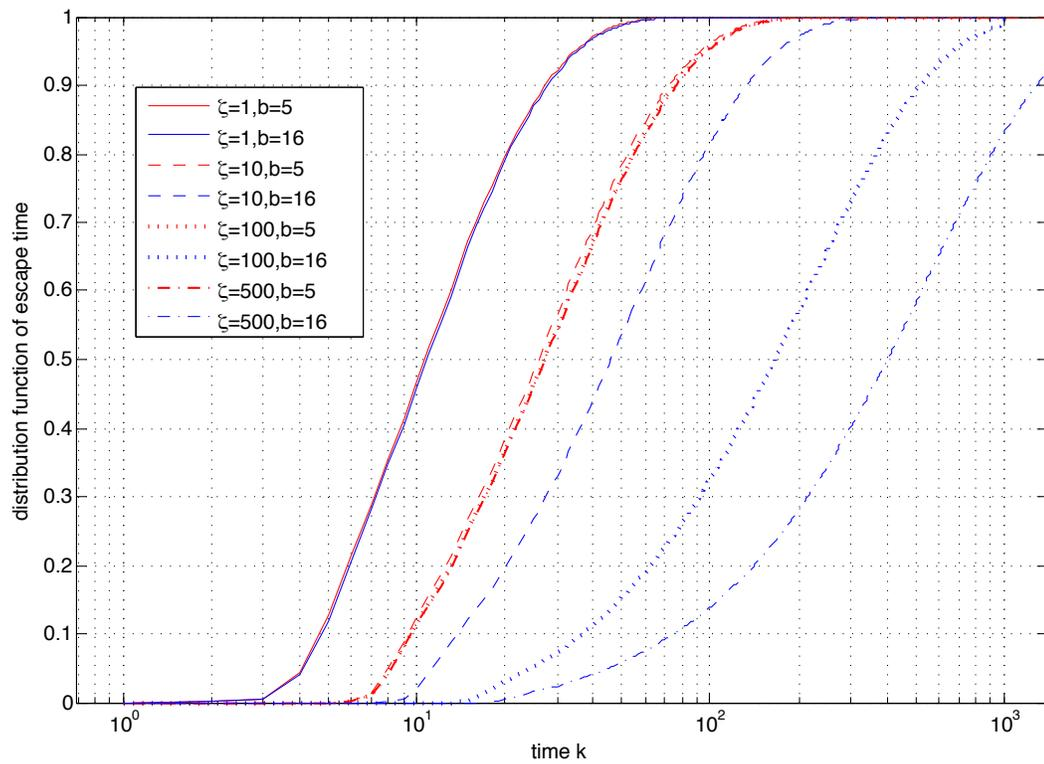
**Figure 4.5.** Cumulative distribution functions of controlled output escape times for Example 1 with  $\zeta = 1, 10, 100, 500$ , and with  $P_\gamma = 0.2$ . Results are shown for 5-bit quantization (red) and 16-bit quantization (blue).
