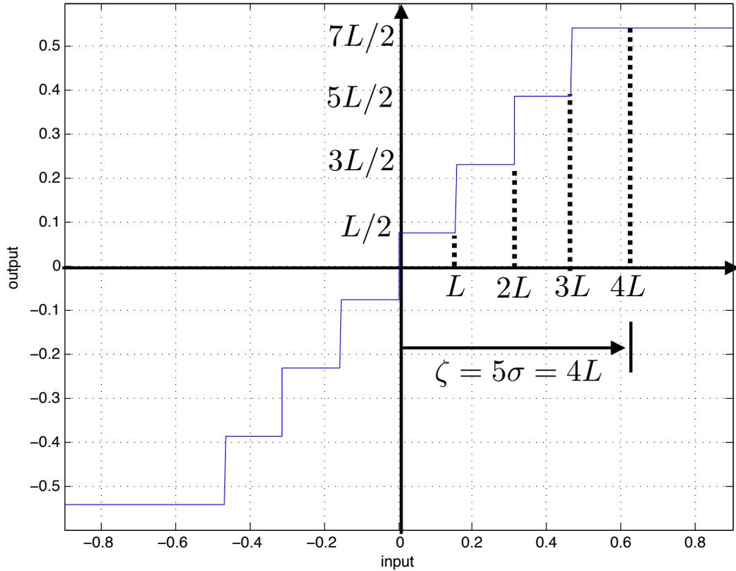
**Figure 5.2.** Quantizer-dequantizer function for Example 6.1. Three-Bit ( $m = 8$ ) uniform quantizer-dequantizer pair input-output relation. The values for this quantizer are based on a steady-state innovations covariance  $\sigma^2 = 0.0155$ .
