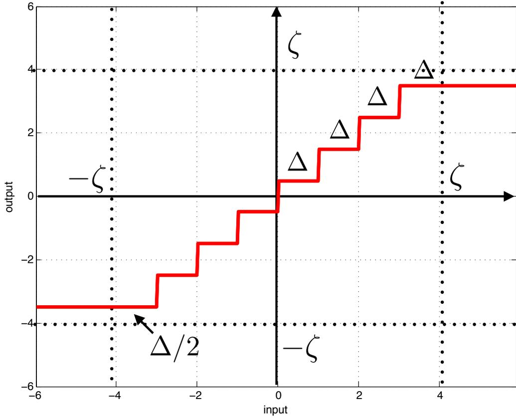
**Figure 2.2.** The linear quantizer  $\Omega$
