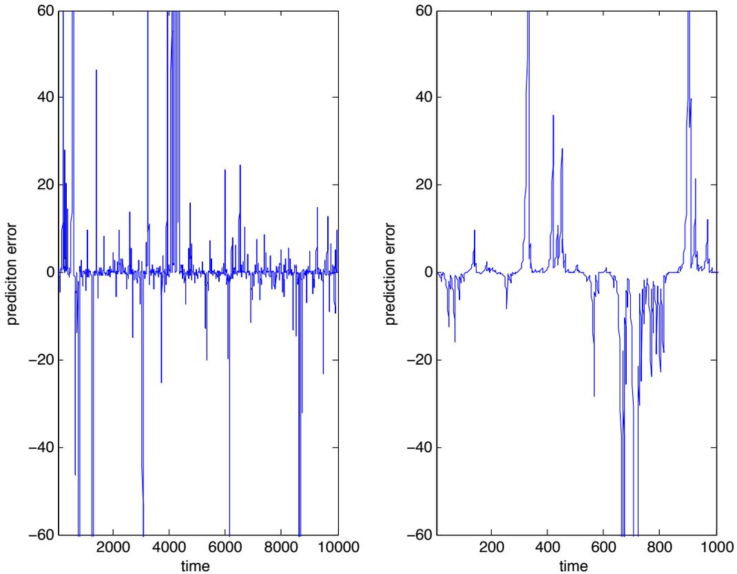
**Figure 1.1.** Simulation of Kalman predictor error with  $A=1.2$ ,  $C = 1$ ,  $Q = 0.005$ ,  $R = 0.001$ ,  $P_\gamma = 0.15$  (left) and  $0.1$  (right), and bound level 60.
