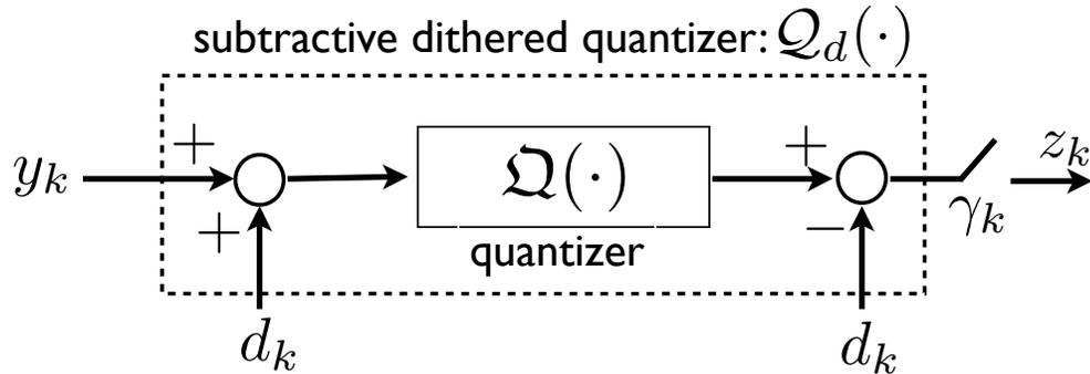
**Figure 2.1.** Subtractive dithered quantization including intermittent gain  $\gamma_k$ .
