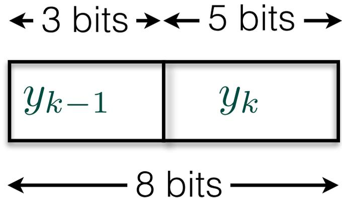
**Figure 4.6.** Bit allocation scheme. Here 3 of 8 bits at time  $k$  are assigned to  $y_{k-1}$  and 5 bits to  $y_k$ .
