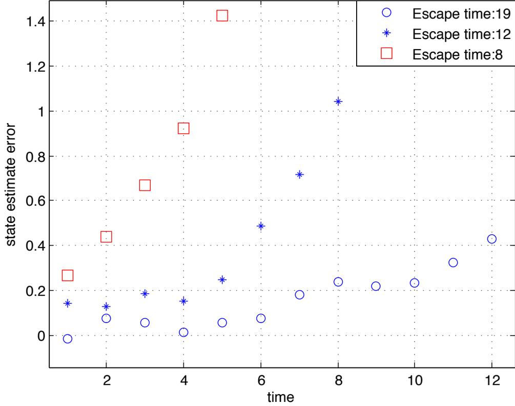
**Figure 4.2.** Three different estimator survival time trajectory samples for Example 1 with initial error covariance  $\Sigma_{1|0} = 0.00725$ .
