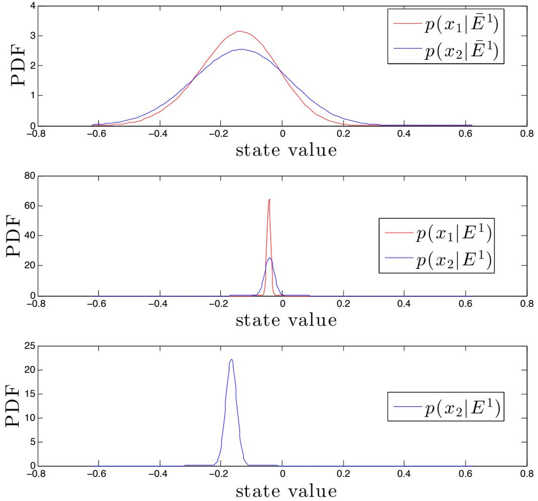
**Figure 6.4.** The estimation quantities:  $\hat{x}_{2|1} = -0.0410$ ,  $\Sigma_{2|1} = 0.0156$ ,  $\hat{x}_{2|1}^{SOI} = -0.1661$ ,  $\Sigma_{2|1}^{SOI} = 0.018$ . The signal values in the transmitter-side system are:  $x_1 = -0.1260$ ,  $x_2 = -0.2286$ ,  $w_1 = -0.1089$ ,  $v_1 = 0.1117$ .
