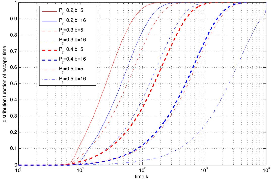
**Figure 4.4.** Semilog plot of cumulative distribution functions of output escape times for 5-bit (red) and 16-bit (blue) quantized measurements as the probability of successful packet arrival,  $P_\gamma$ , varies.
