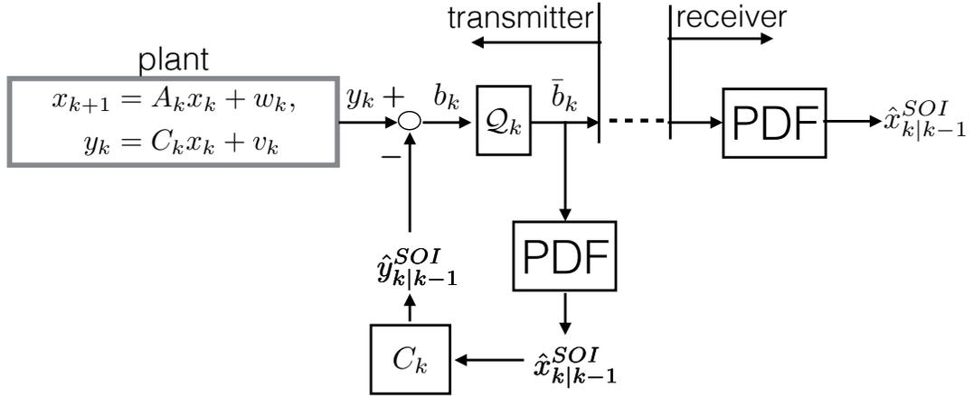
**Figure 5.3.** Block diagram representation of the Bayesian filtering approach of [2], where the transmitter replicates the receiver's computation of the predicted states conditional pdf to calculate an innovations signal for quantized transmission.
