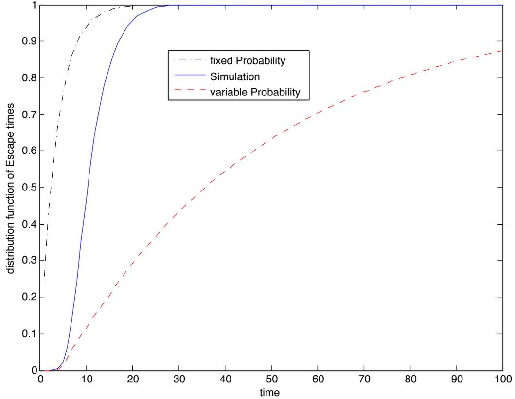
**Figure 4.3.** Comparison of escape time cdf for Sinopoli's Example: unbroken curve – simulation, dash-dot curve and dashed curve are both using (4.1) with fixed expected condition covariance or time-vary conditional covariance then averaged over 1000 trials.
