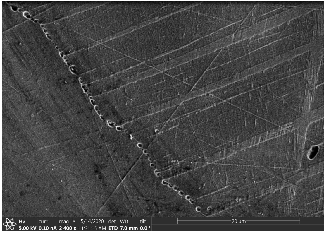
Figure 3.22 Grain boundary precipitates in deformed hat shape specimen after etching.
