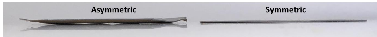
Figure 7. Symmetric cells are flat. Edge-on photograph of 50 cm 2 (left) asymmetric cell (metal/porous ceramic/dense ceramic/porous ceramic) and (right) symmetric cell (metal/porous ceramic/dense ceramic/porous ceramic/metal) after identical sintering processing.
