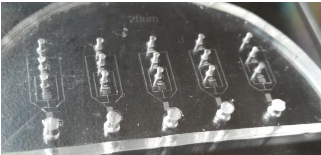
Figure 6: Photo of finished device fabricated via Peel Method. Contains 5 individual devices.
