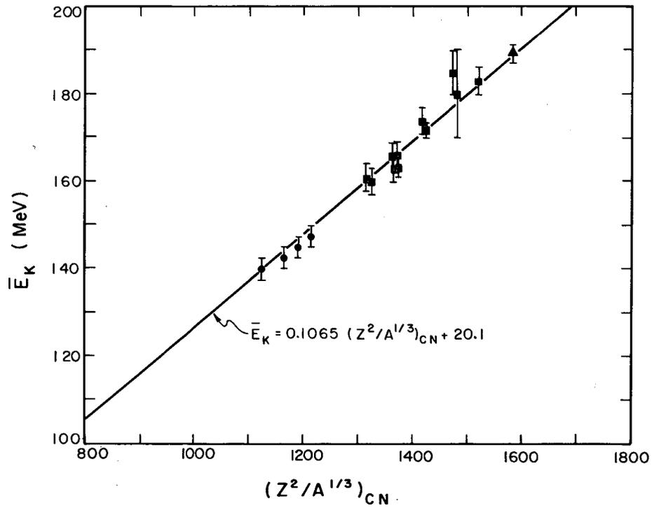
Fig. 4. Plot of  $\bar{E}_K$  versus  $Z^2/A^{1/3}$  for data obtained elsewhere. Squares (■) represent results from reference 3; circles (●) are from reference 20, and the triangle (▲) is from reference 21.
