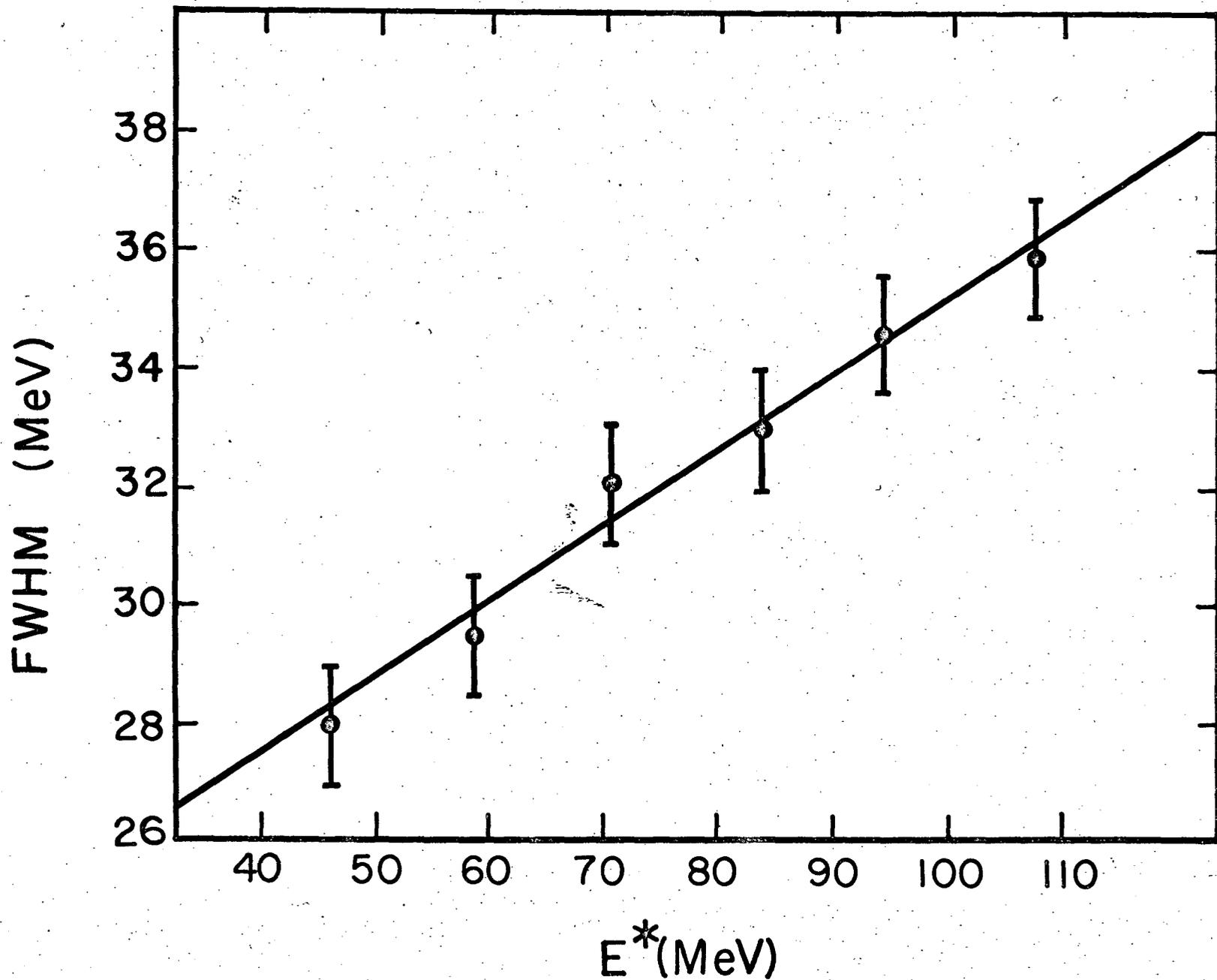
Fig. 11. Full-width at half maximum of the fission fragment kinetic energy spectrum for bombardment of  $\text{Bi}^{209}$  with  $\text{O}^{16}$  ions at several excitation energies.
