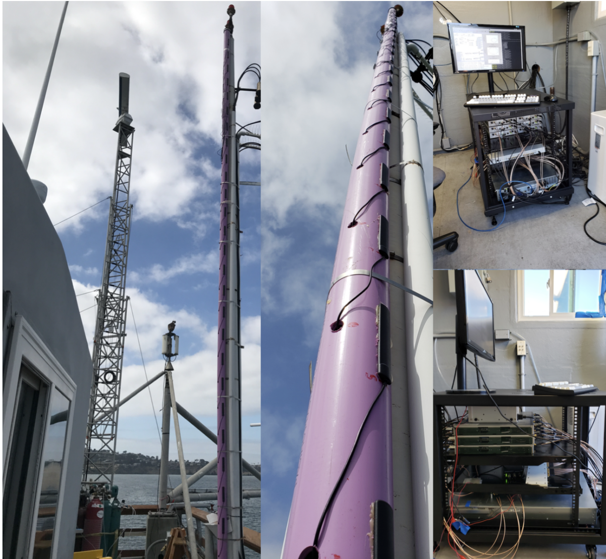
Figure 5.2: Coherent receiver array positioned on the end of Scripps Pier and control station setup inside nearby shed.
