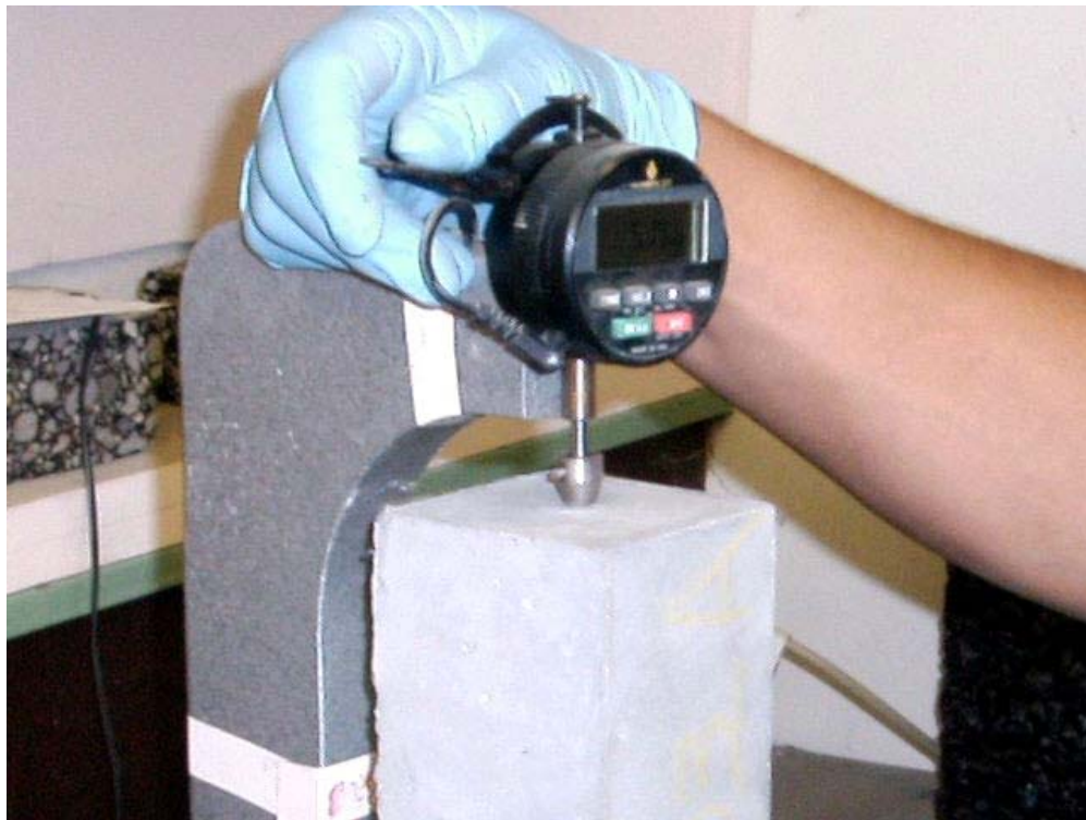
Figure 2.6. Shrinkage test configuration.
