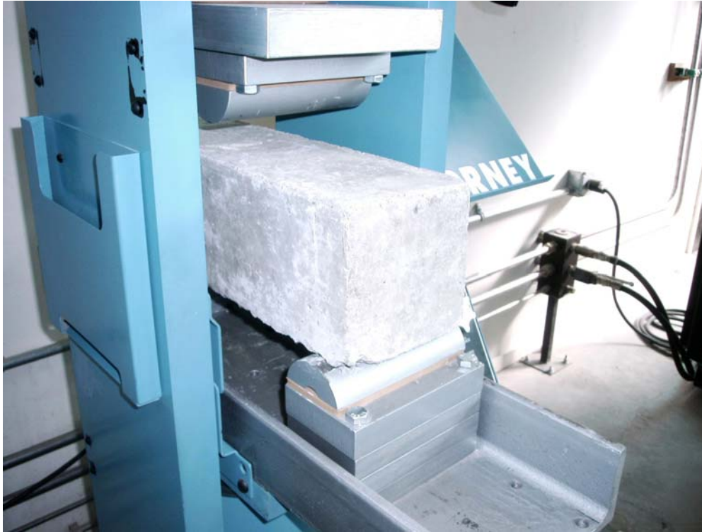
Figure 2.4. Flexural test configuration.
