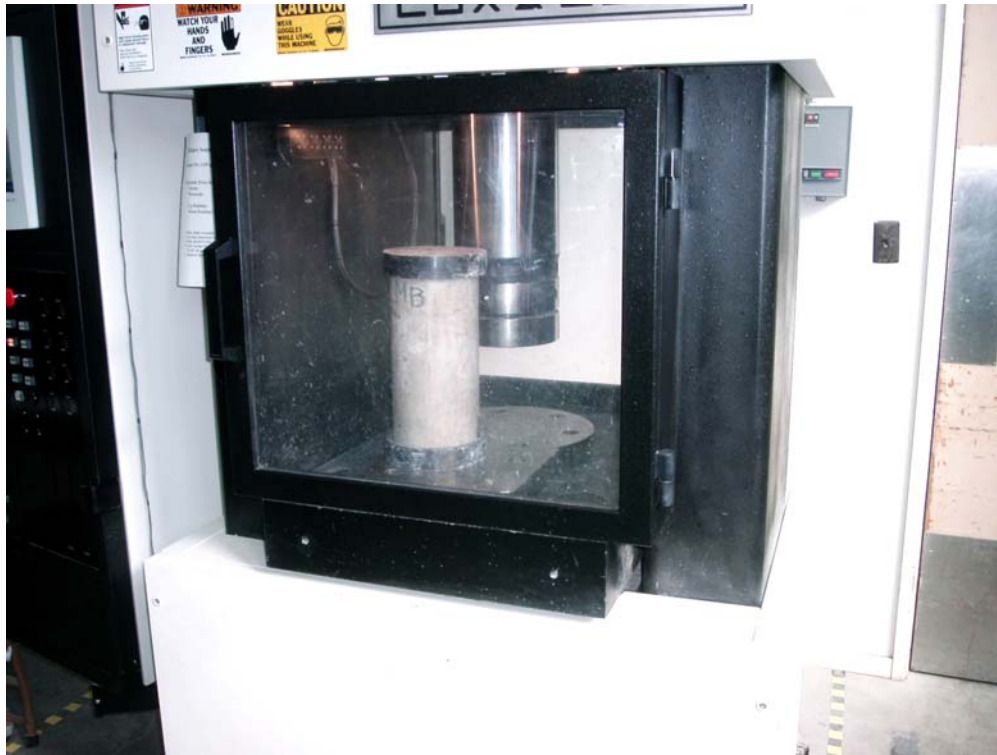
Figure 2.5. Compressive strength test configuration.
