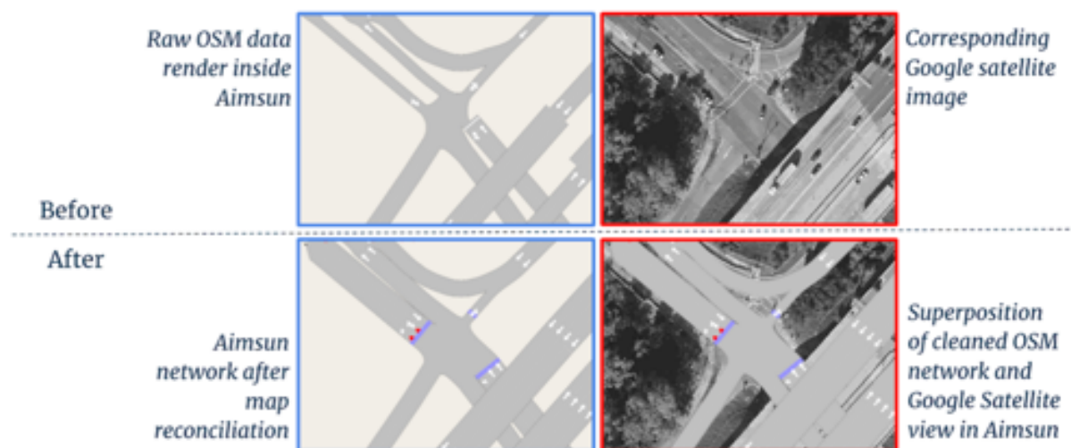
Figure 5.2: An intersection of the Aimsun network before and after manually editing the OSM network using Google Satellite images.
