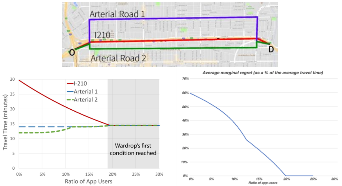
Figure 3.2: On top: Benchmark network. At the bottom: The path travel times (on the left) and the average deviation incentive (on the right) as a function of the percentage of app usage. On the benchmark network, the traffic converges to a user equilibrium state when app usage increase. Figure reproduced from [47, Figure 3].
