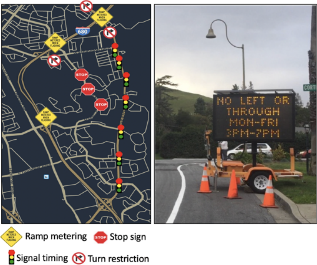
Figure 2.5: Left: Traffic-calming strategies implemented by the city of Fremont to decrease traffic on local roads due to commuters' cut-through. Right: An illustration of the Fremont turn and access restriction during evening peak hours.
