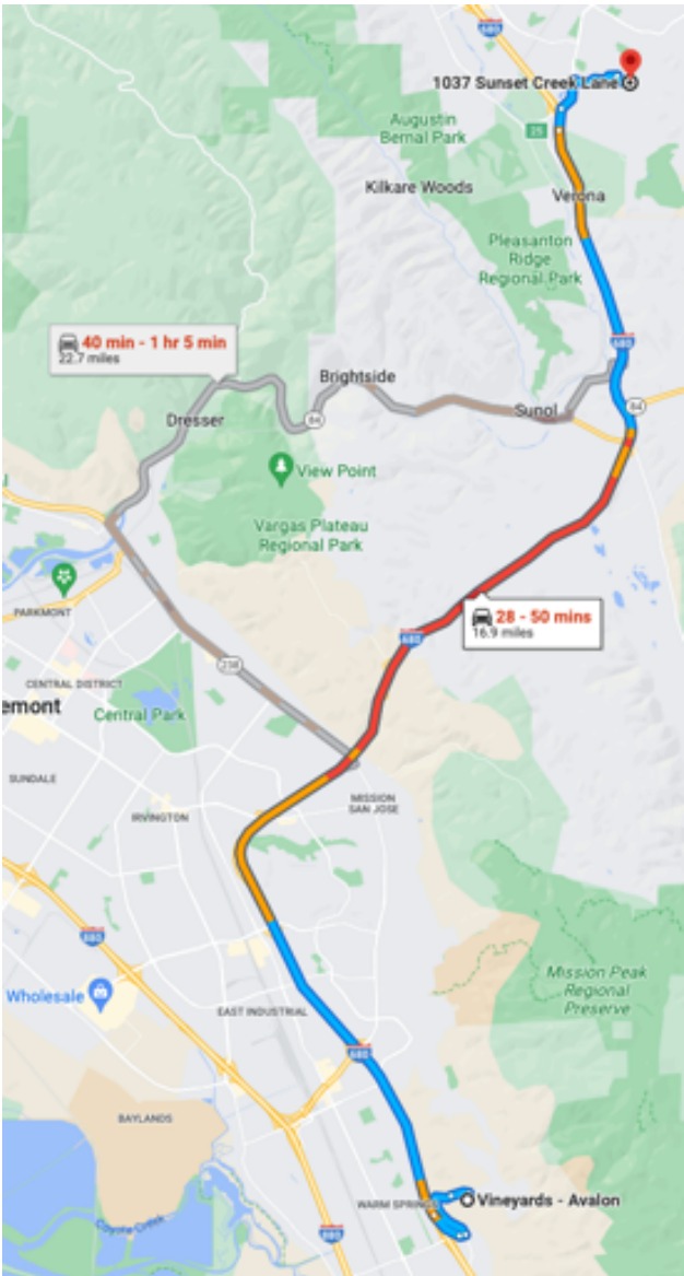
Figure 2.8: July 14 th , 2022 4:30 pm, traffic guidance on Google Maps within the Fremont, CA area. The request is done on July 13 th and uses the Google Maps traffic prediction system. The first route suggested (in blue, orange, and red) uses a local road, then a collector road, then a minor arterial road, and then an interstate before using a minor arterial, a collector, and then a local road to reach its destination. The road categories of the road used by the trip increase and then decrease. However, in the second road suggested (in grey), this is not the case: a major arterial, a minor arterial, and a collector road are used between the same interstate road.
