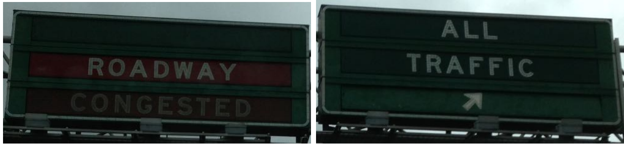
Figure 2.6: One of the first Variable Message Signs (VMS) on the New Jersey turnpike in the 1950s. Variable message signs were the first tools to manage route choice in real-time without the need of a traffic police agent, or temporary road signs. Nowadays, we envision that eventually variable message signs will be overridden by navigational apps or any other connected devices.
