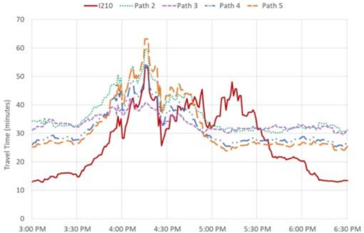
Figure 4.4: Evolution of travel times on the paths parallel to the I-210 considered (fig. 4.3) on March 10 th , 2014. At the beginning and end of the peak hour (3-6 PM), the travel time on the freeway is close to the free flow travel time, and the freeway is faster than the arterial routes. However, when the freeway travel time increases, arterial detours become beneficial alternatives. During high congestion, drivers can reroute themselves to arterial roads to reduce their travel time, leading to travel time equalization among parallel routes. The figure is reproduced from [48, Figure 3].
