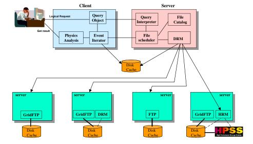
Fig. 1. A scatch of the Grid Collector.
