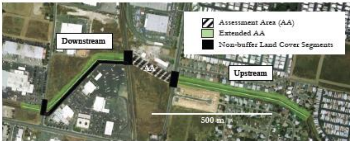
Figure 4: Diagram of method to assess Stream Corridor Continuity of riverine wetlands. This example shows that about 400 m of “non-buffer land cover” disrupts the stream corridor within 500 m downstream of the AA. This is due to the large parking lot that impinges on the south side of the stream in addition to two bridge crossings that disrupt the buffer on both sides of the stream. There is a 10 m non-buffer segment in the stream corridor upstream of the AA due to a bridge crossing (10 m for each side of the stream, adding up to a 20 m break total). The upstream segment of the stream has an intact stream corridor (green stream reach) upstream from the AA, except for the bridge directly upstream (black area).
