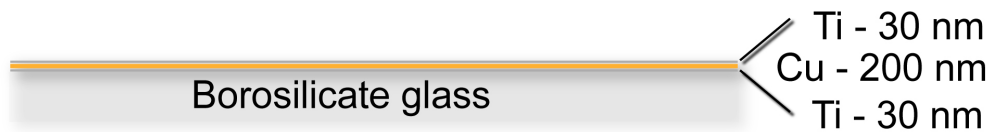
Figure 3.6: Step 1: We begin with glass slides (purchased from Fisher Sciences), which are cut in half, and cleaned in piranha and oxygen plasma (Tegal Asher, 200 W, 5 min). Ti/Cu/Ti seed layer is deposited to thicknesses of 30 nm / 200 nm / 30 nm in a CHA evaporator.
