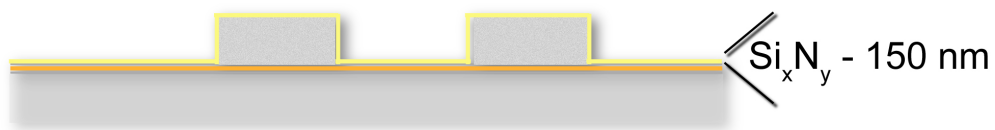
Figure 3.9: Step 4: KMPR electroplating mold is stripped in Aleg-355 or Aleg-380 photoresist stripper over 30 minutes at 75 C. The seed layer is etched first in 1 % hydrofluoric acid, then in 5 % acetic acid / 15 % hydrogen peroxide, and again in 1 % hydrofluoric acid. The metal layer is finally passivated with 150 to 200 nm of PECVD \text{Si}_x\text{N}_y at 300 C.
