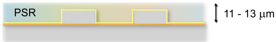
Figure 3.10: Step 5: For our force substrates, PSR resist is spun with a ramp of 500 rpm/s, baked under ramping conditions for 20 minutes from 65 to 95 C, 55 second exposure dose, hard baked for 6 minutes at 95 C, and cured at 120 C for 12 minutes.
