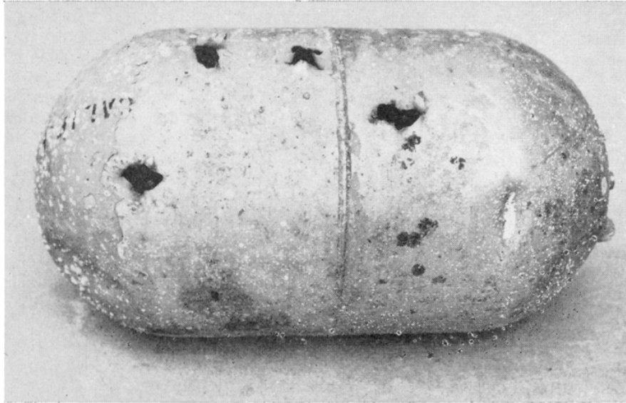
FIGURE 8. Metal buoy used to mark artificial reef shot full of holes and sunk by vandal. Photograph by Jack W. Schott, April 1962.
