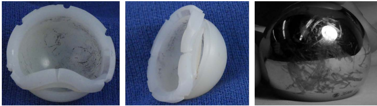
Figure 2.15 | Fractured highly crosslinked UHMWPE liner and CoCr femoral head. The left image shows mild pitting and scratching damage, highlighted using black ink, as well as the exposed surface of the fractured rim below. The middle image shows another perspective of the fracture. On the right, the CoCr femoral head exhibits several large scratches along the distal slope.
