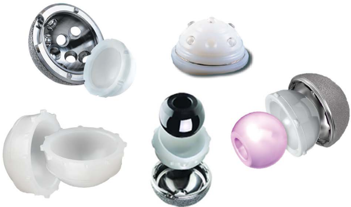
Figure 2.14 | A few of acetabular liners currently on the market. Each liner contains design features (notches) that enable liner fixation within a metal acetabular shell. These liner locking mechanisms have demonstrated enhanced fixation that reduce backside wear and liner dissociation; however, each mechanism includes notches that serve as stress risers where cracks can form and propagate. (Zimmer 2014a; Zimmer 2014b; Depuy 2013; Smith & Nephew 2014; Pierson 1995)
