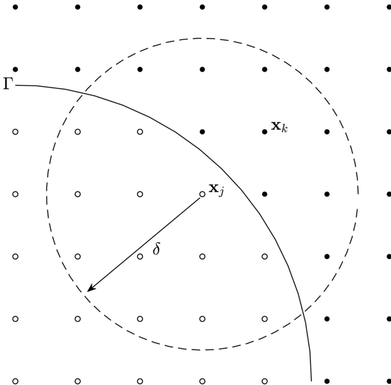
**FIG. 3.** Illustration of a scaled kernel centered at the center  $\mathbf{x}_j$  of a grid cell and vanishing outside a sphere (indicated by the broken lines). Black dots represent centers of grid cells in the solvent region  $\Omega_w$  and circles represent the centers of grid cells in the solute region  $\Omega_m$ .
