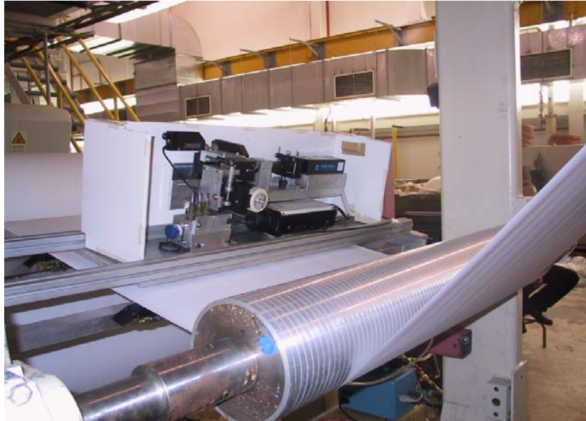
Figure 3. LUS system installed on pilot coating machine.
