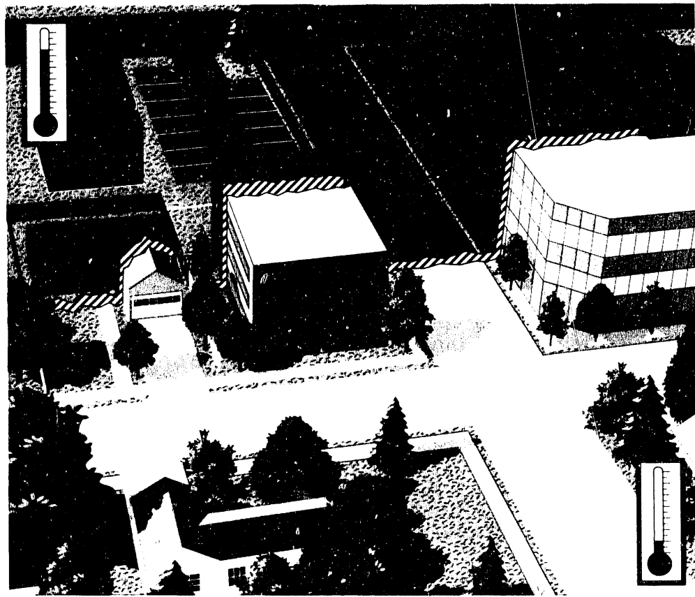
Figure 3-2. Surface contrast. Simply changing the surface colors of our urban communities could significantly decrease their temperatures.
