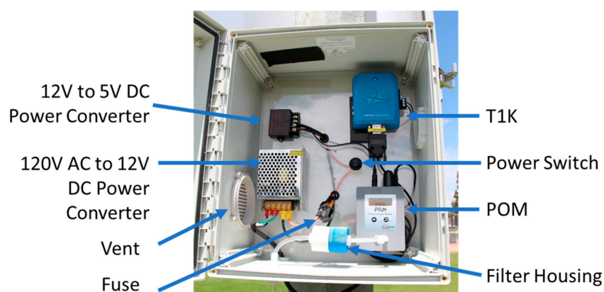
Figure 1. Ozone sensor node with labeled components.
