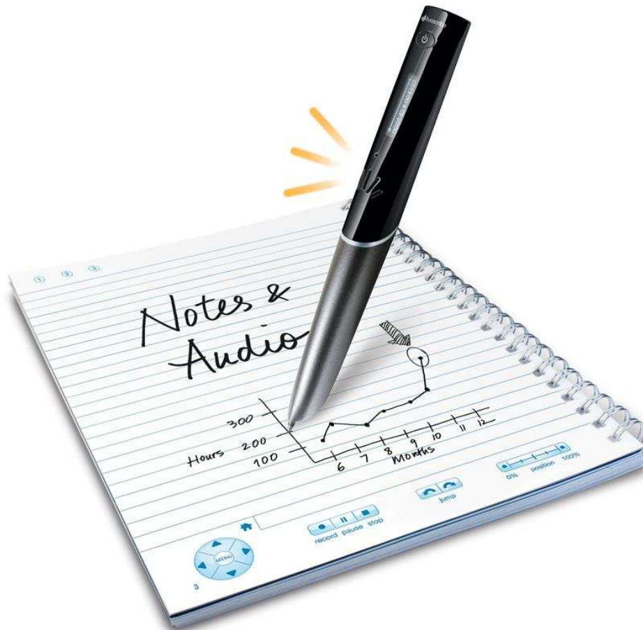
Figure 3.1: The Livescribe™ digital pen. This pen allows users to write ink on paper, but additionally digitizes the writing, producing a time-stamped record of the ink. This technology is enabled by the special Anoto™ paper on which the user must write. This paper comprises a tiny dot-matrix pattern which a tiny camera, located near the tip of the digital pen, uses to determine where on the page the pen is writing.
