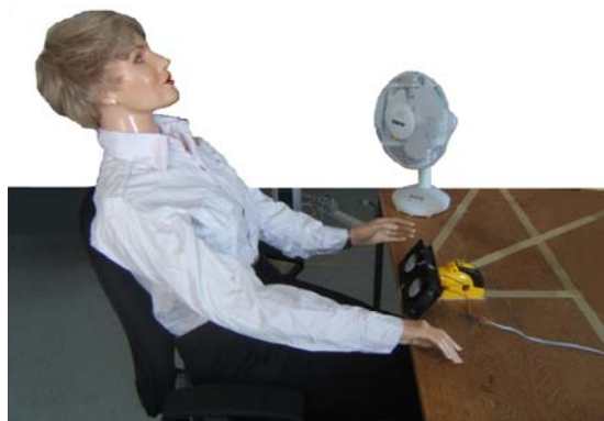
Figure 1. The desk fan, the two computer fans and the thermal manikin, and their location relative to the thermal manikin.
