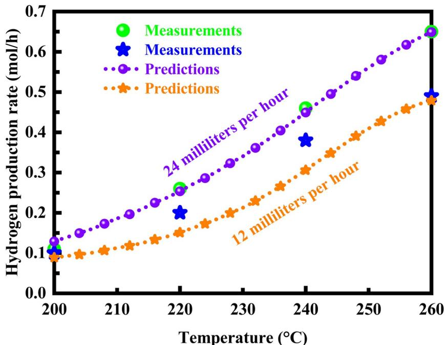
Figure 2. Effect of reaction temperature on the rate of hydrogen production. The data obtained by measurements are also presented to validate the model.
