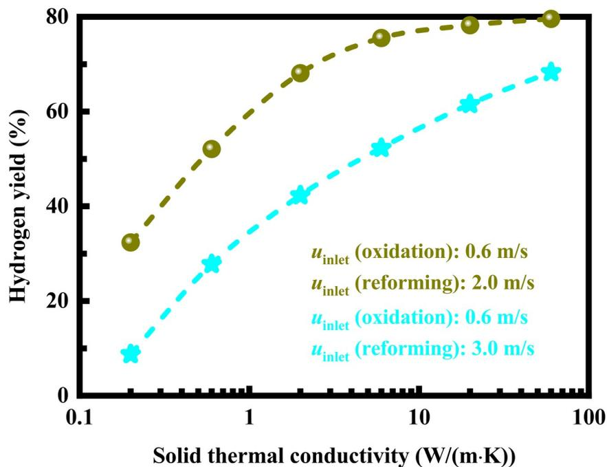
Figure 6. Effect of solid thermal conductivity on the hydrogen yield of the microchannel reactor at different inlet gas velocities.
