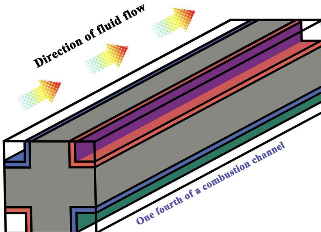
Figure 1. Schematic representation of the computational domain of the complex reactor for producing synthesis gas by steam-methanol reforming.
