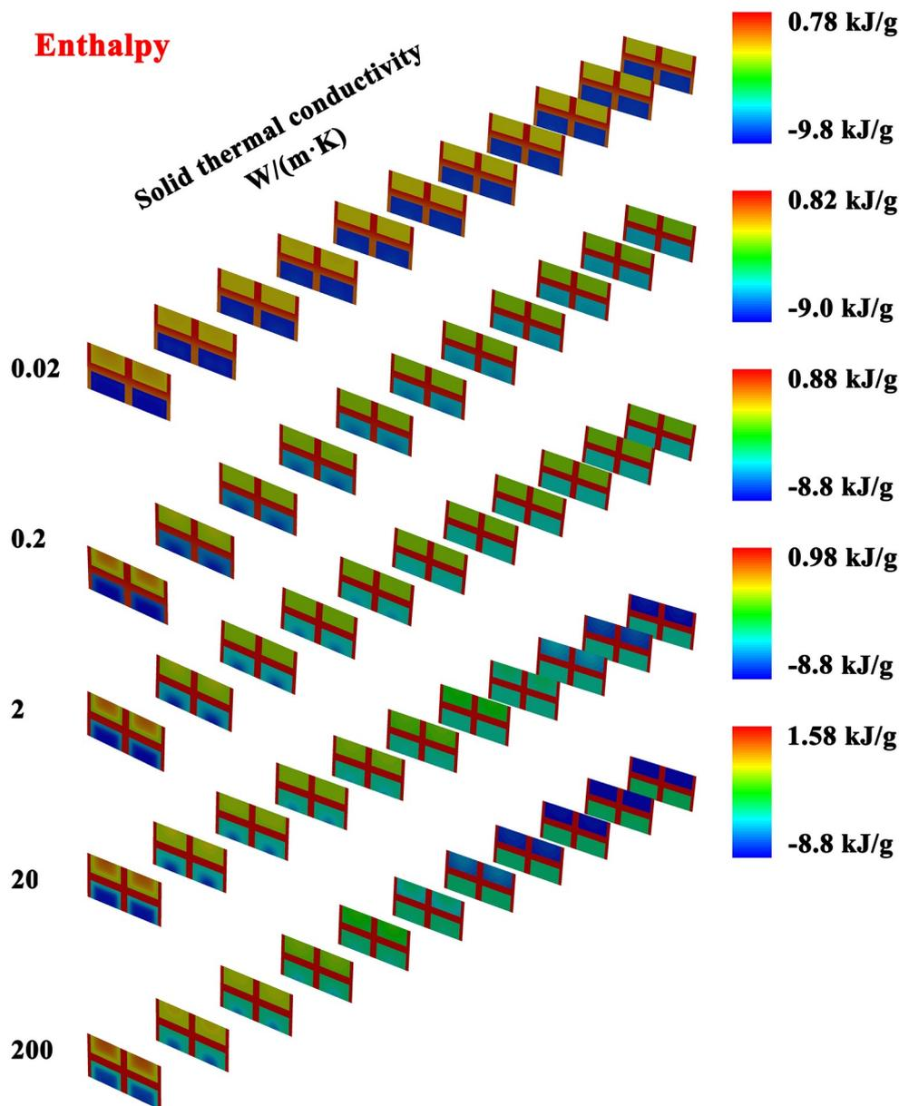
Figure 5. Enthalpy contour maps in the reactor with different solid thermal conductivity. The reactor walls are constructed of stainless steel.
