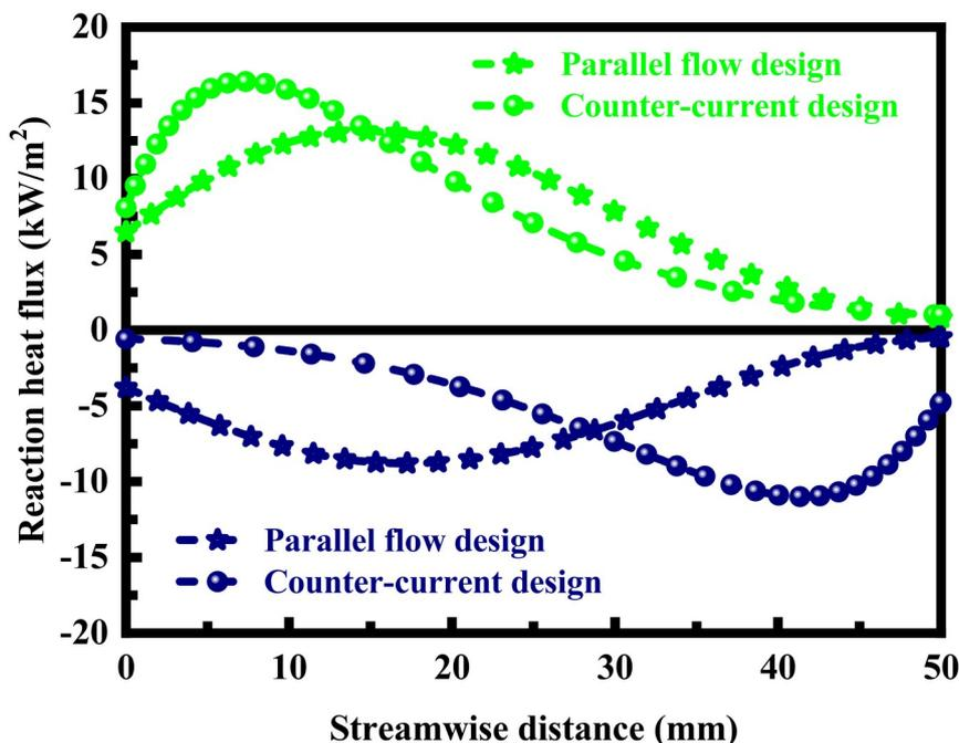
Figure 9. Effect of flow arrangement on the heat fluxes of the oxidation and reforming reactions in the reactor. The heat flux results are presented for the parallel flow design and for the counter-current design.
