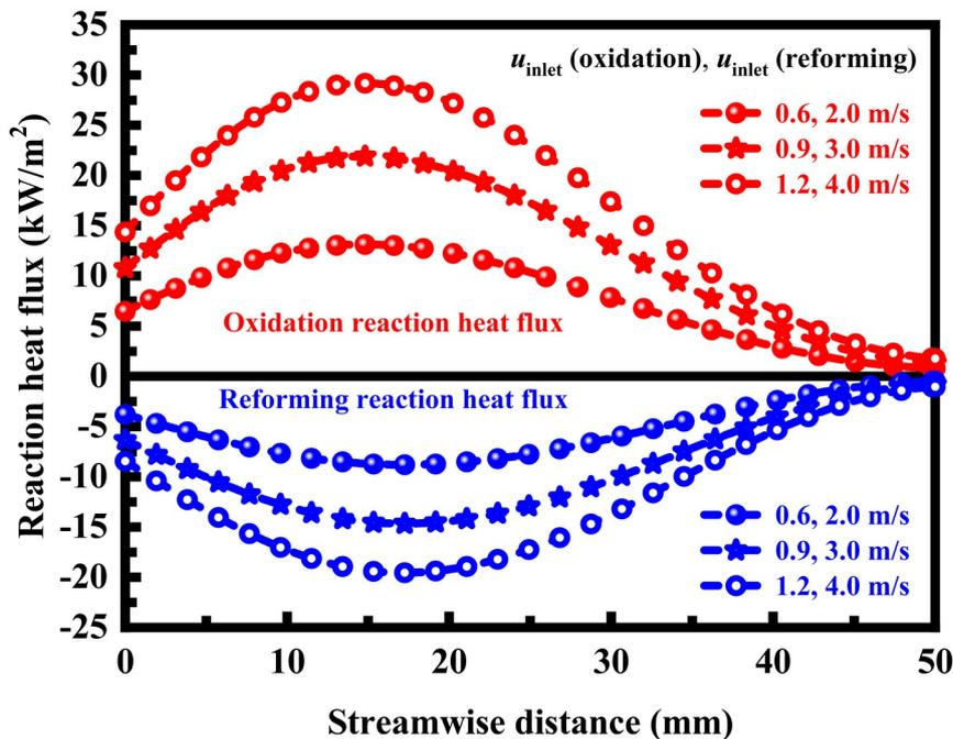
Figure 4. Effect of the gas velocity at the channel inlets on the heat fluxes of the oxidation and reforming reactions in the reactor.
