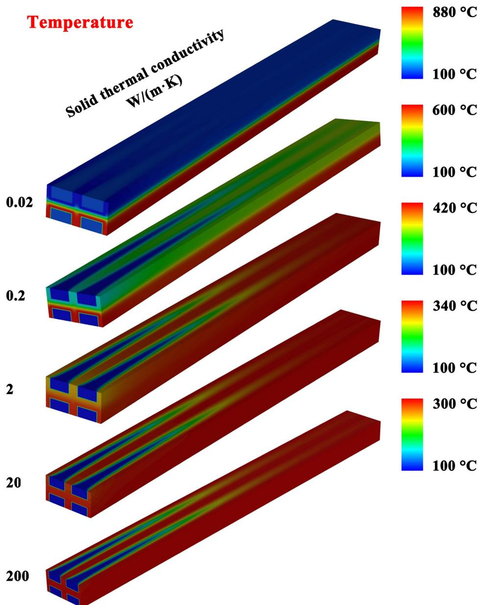
Figure 3. Temperature contour maps in the microchannel reactor with different solid thermal
