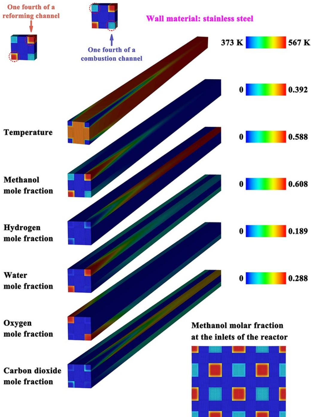
Figure 8. Species mole fraction contour maps in the microchannel reactor when the reactor walls are constructed of stainless steel.
