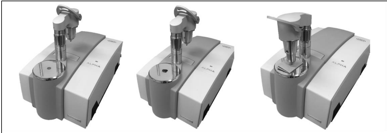
Figure 4.5: Application of sample: FTIR device before sample loading (left), with attached sample (center) and with paper spacer and holding arm (right).
