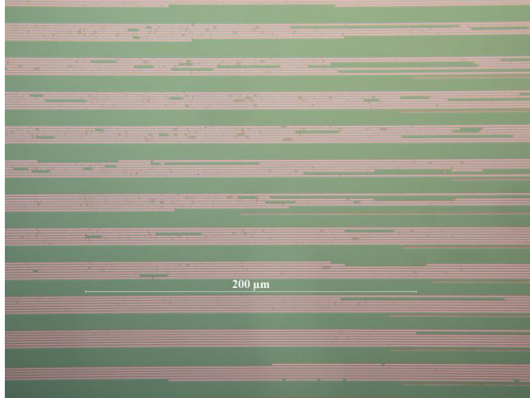
Fig. 66. A set of 10^{18} \text{ cm}^{-3} n -doped GaAs nanoribbon ( L/W/T = 400/0.75/0.03 \text{ }\mu\text{m} ) arrays transferred to \text{SiO}_2/\text{Si} . Each individual array is nominally composed of ten parallel ribbons. Discontinuities along the nanoribbons indicate broken segments resulting in <100\% yield.
