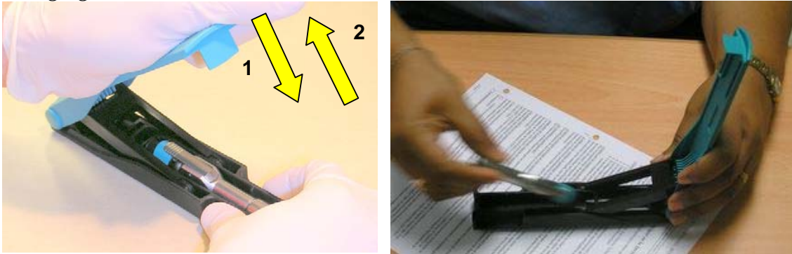
Figure A-16. (Left) The device is charged by loading the device in the charging box, (1) closing the lid, and then (2) opening it. (Right) Subject loading the device into the charging box.
