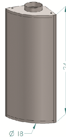
Figure 3. Displacement diffuser used in the room. Dimensions in inches.
