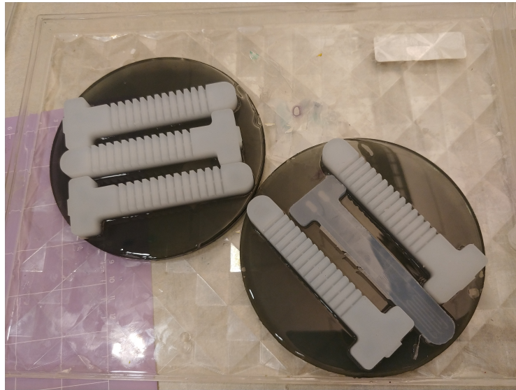
Figure 2.9: This figure shows multiple actuator pieces being glued to a silicone "skin". Once cured they will be cut out of the skin and can then be attached to other pieces to form a complete actuator.
