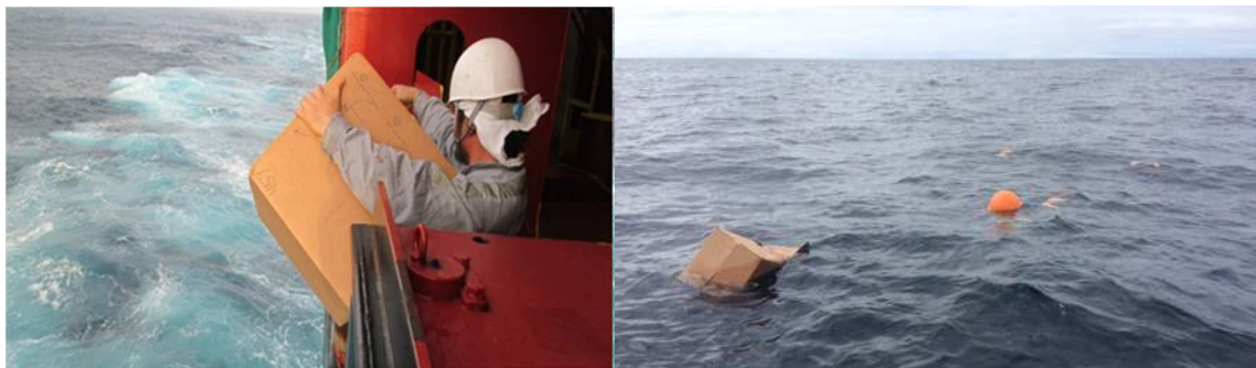
Figure 3: Wave buoy deployed off the APL container ship in 2016. The buoys use alkaline batteries and are packaged in cardboard boxes to allow for ease of shipping and deployment.
