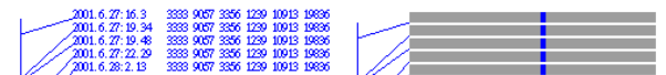
Figure 4: Oscillation is defined as closely-spaced consecutive announcements alternating between two unique paths.
