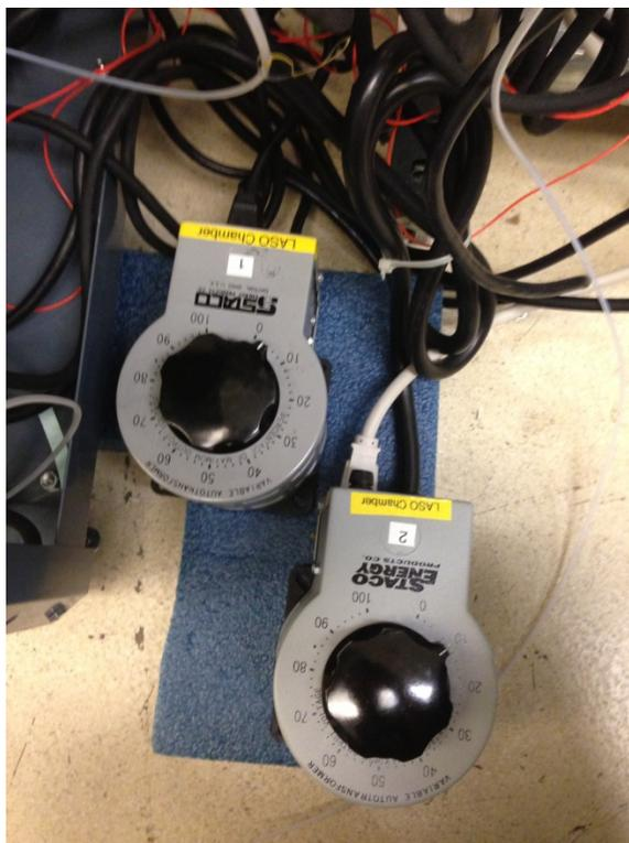
Figure B11. Transformers for the sample stage heater and dosers
