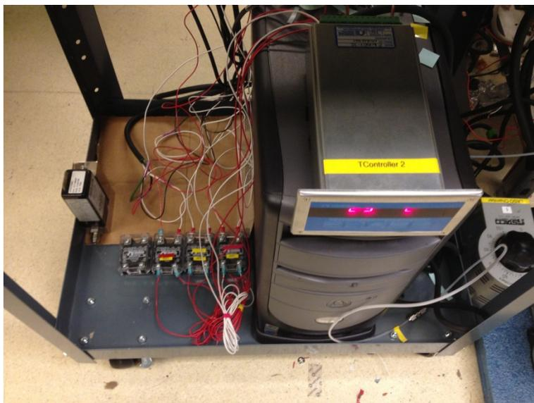
Figure B12. Temperature Controller 2 and Solid-state Relays
