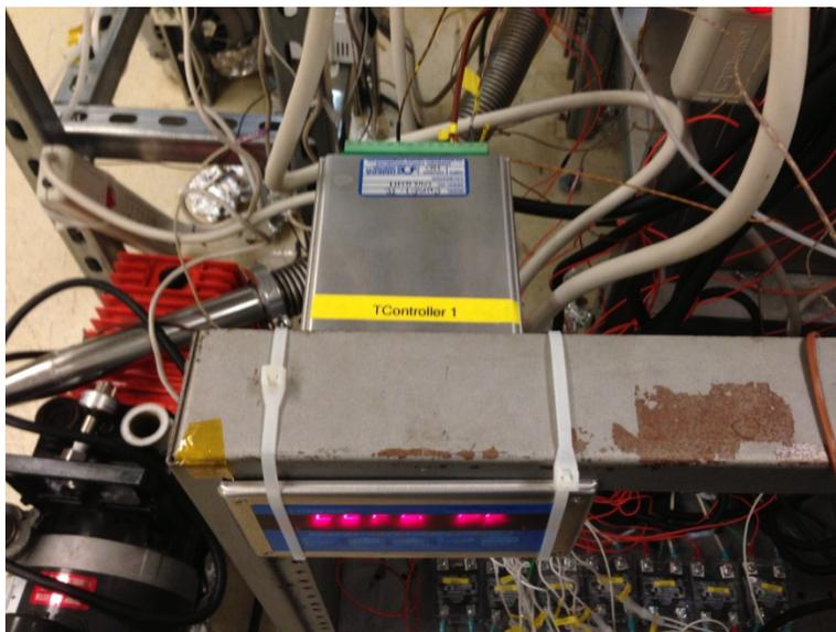
Figure B10. Temperature Controller
