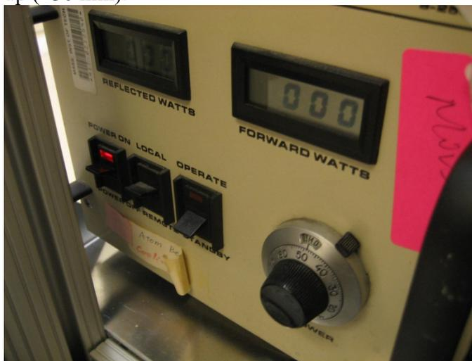
Figure A5. Microwave Power Source. Power switch (left), Operate/Standby switch (middle). Power control knob (right)
