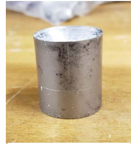
Figure 12: 45° die with cracks in the body of the die.
