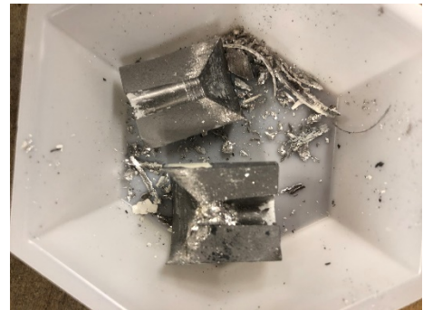
Figure 11: Fracture 45° die with back relief. Scraps of billet and die surround the fractured ..
