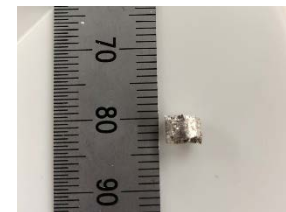
Figure 13: Test 5 extrusion results. a) 90° die after extrusion. b) 3.5mm extrudate with scale bar.
