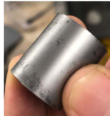
Figure 9: Crack running alongside of the 45° die found after test 1.
