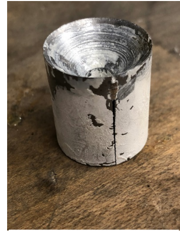
Figure 10: 45° die with back relief coated in boron nitride spray. Further crack propagation present in the side of the die.
