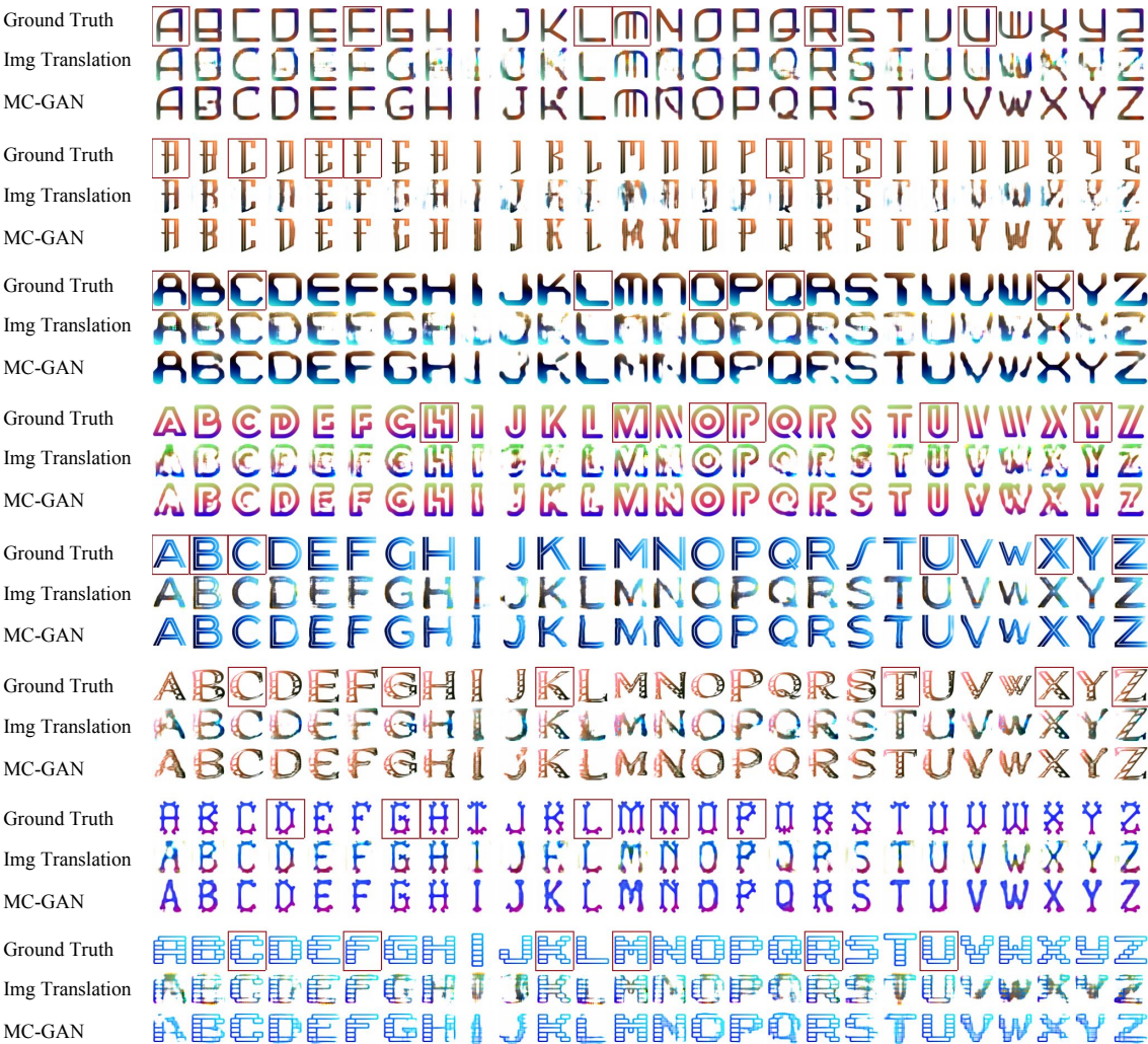
Figure 2.14: Comparison between image translation and our end-to-end multi-content GAN on our synthetic color font data set. For each example, ground truth and given letters are shown in the 1st row , image translation outputs in the 2nd row and MC-GAN in the last row .
