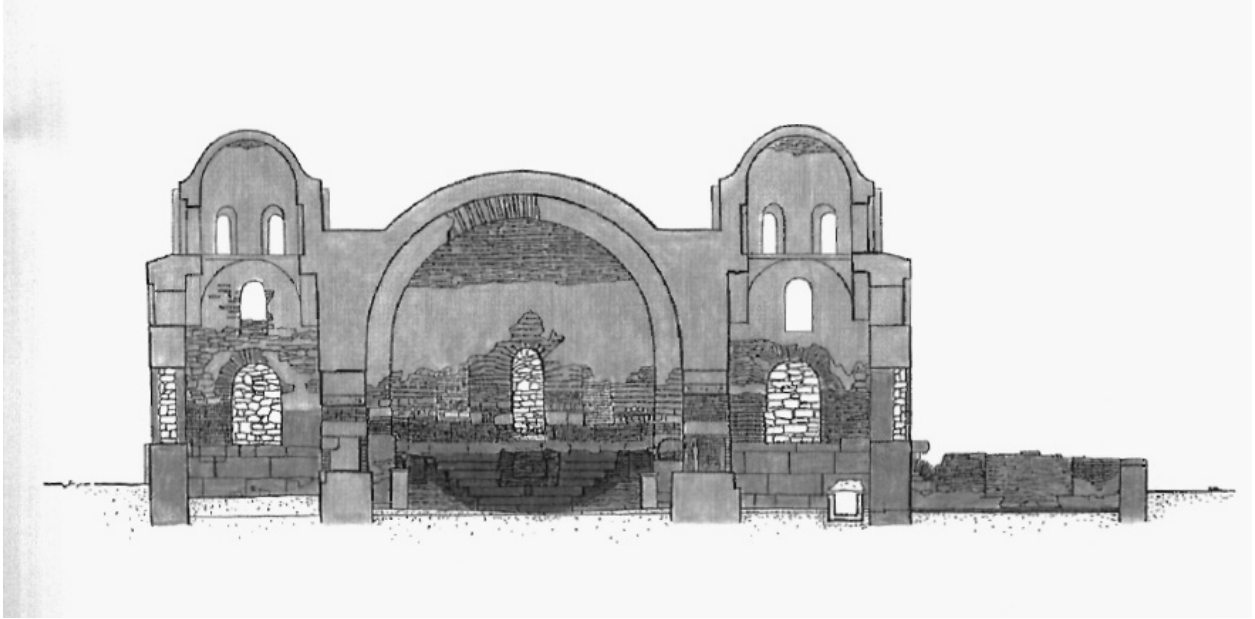
Figure 74: Pastophoria and Apse, East End, Hagia Sophia, Nicæa (from Möllers, Die Hagia Sophia , Beilage 10)
