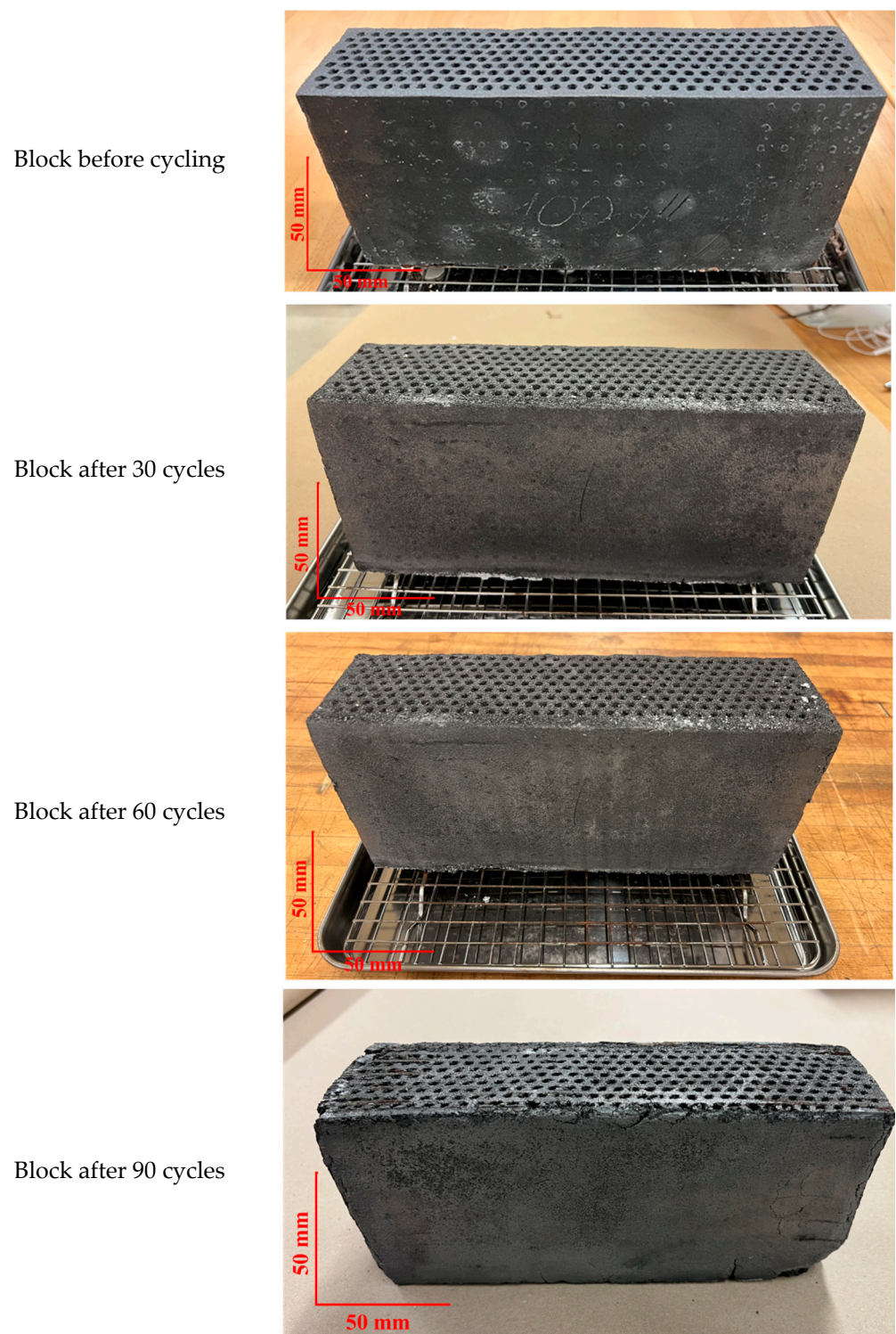
Figure 11. Composite \text{CaCl}_2/\text{EG} perforated block during cycling in the reactor.
