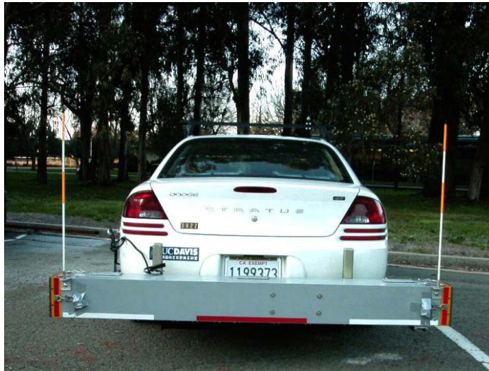
Figure 4: Laser profilometer beam.
