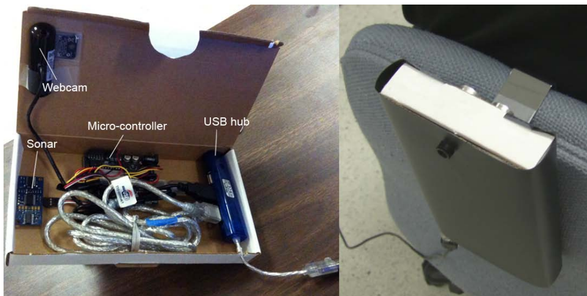
Figure 4.6: Portable sensor box configuration
