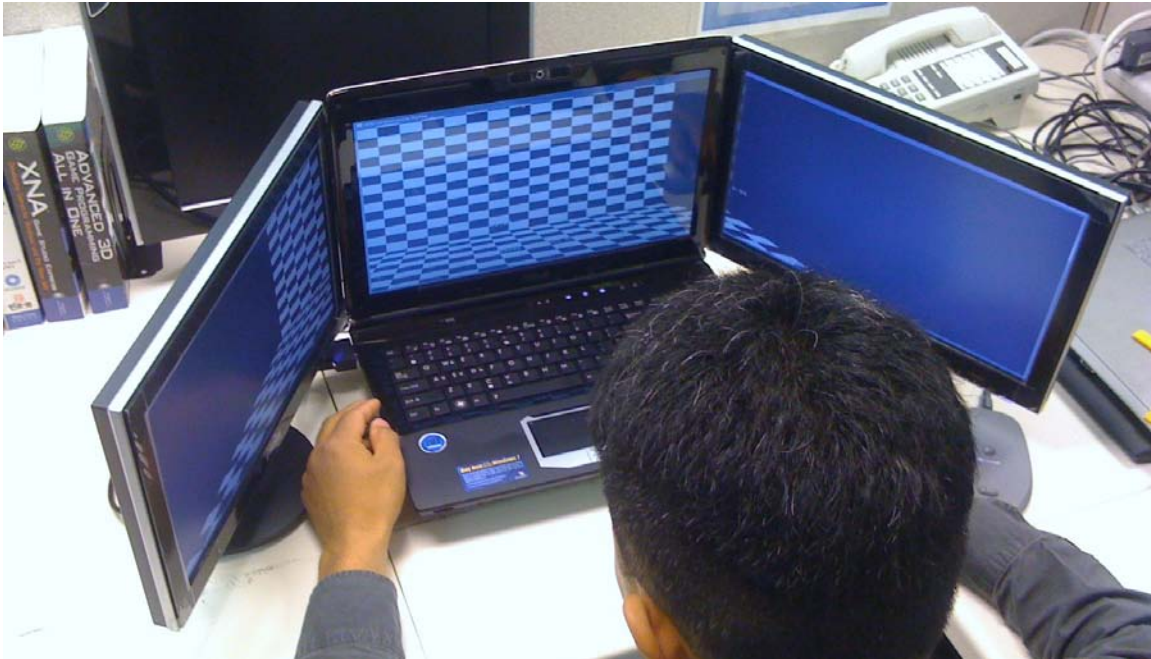
Figure 3.5: A prototype vertical non-planar display with three monitors
