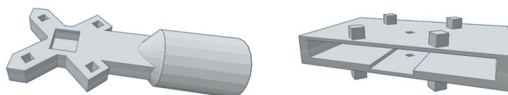
Figure 5.3: Illustrations of 3D-printed modules for (left) the PMT-scintillator assembly and (right) an example phone: the Samsung Galaxy S6.
