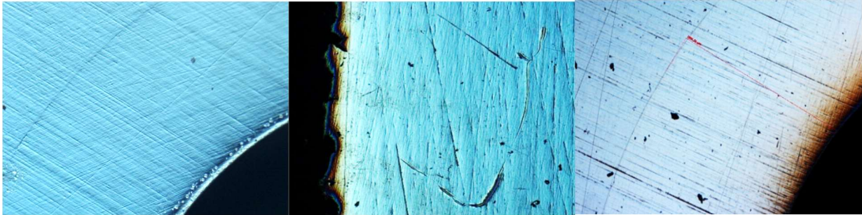
Figure 3-15: 10x Magnified, samples where tube was expanded Control (Left) 6-week (center) 2-week (right)
