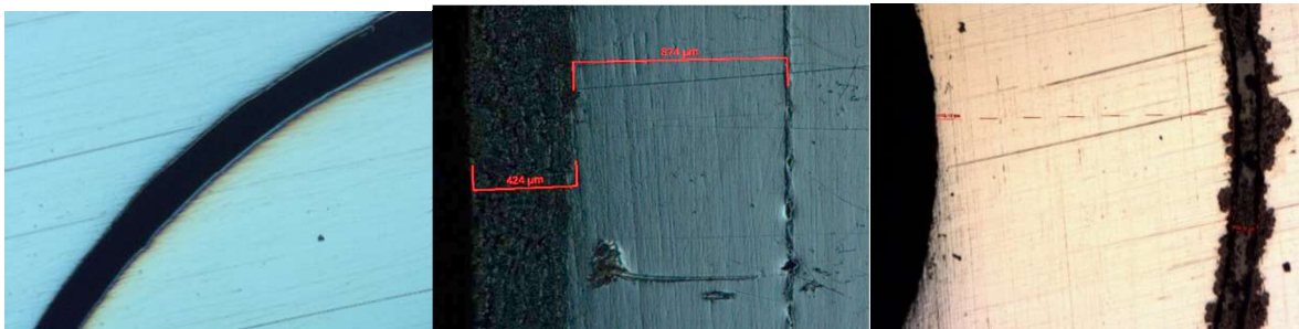
Figure 3-14: 5x Magnified, samples where tube was not expanded. Control (Left) 6-week (center) 2-week (right)
