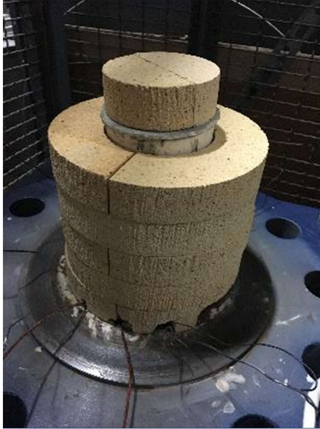
Figure 3-7: Firebrick insulation surrounding alumina tube
