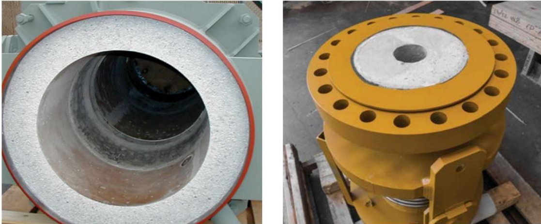
Figure 2-6: Internal insulation in carbon steel pipe[30]
