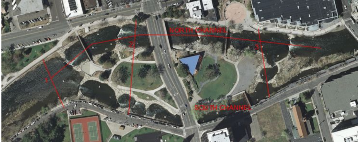
Figure 7: Map of Wingfield Park showing the 3 cross sections surveyed and the surveyed north channel longitudinal profile. Imagery sourced from Google.
