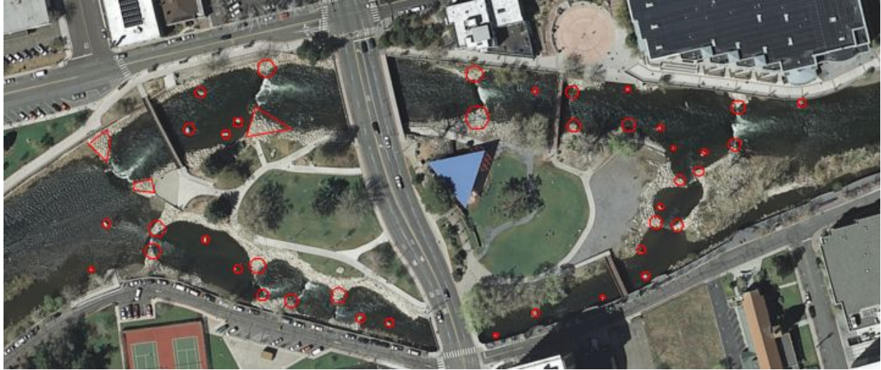
Figure 25: Facies Map of Post-Project Conditions (taken in 11/2019 by DJI Mavic Pro Drone). Instream rock features are highlighted in red.
