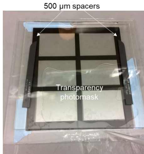
Figure B.1: Gel lid photopolymerization setup. The bottom glass plate is adhered to the transparency photomask which defines the length and width of the gel lid to be photopolymerized, while gel lid height is set by the spacers. Gel precursor solution is pipetted between the glass plates.
