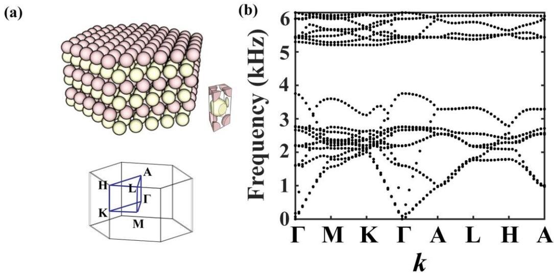
**Figure 5.1 Hcp phononic crystal with a large band gap.** (a) Hcp phononic crystal made with steel metal balls in an epoxy background. The two colors indicate the AB stacking of the hcp crystal. (b) A 3D band gap in the hcp crystal.
