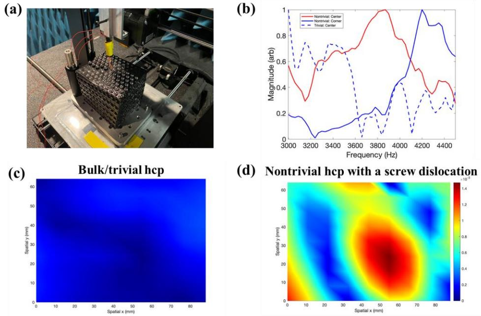
**Figure 5.4 Measurement of the screw-dislocation waveguide.** (a) Measurement setup. (b) Displacement amplitude vs. frequency at the center of the nontrivial sample compared to that at the center of the trivial sample and that at the corner at the nontrivial sample. (c) and (d) are the field scan on the top of the trivial and nontrivial samples at frequencies in the bandgap, respectively.
