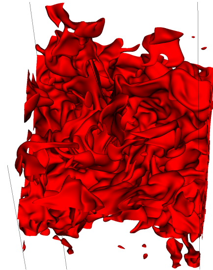
Figure 6. Isosurface (temperature of 1225K) for methane flame data set extracted using our algorithm. The isosurface consists of approximately 29.7 million triangles.
