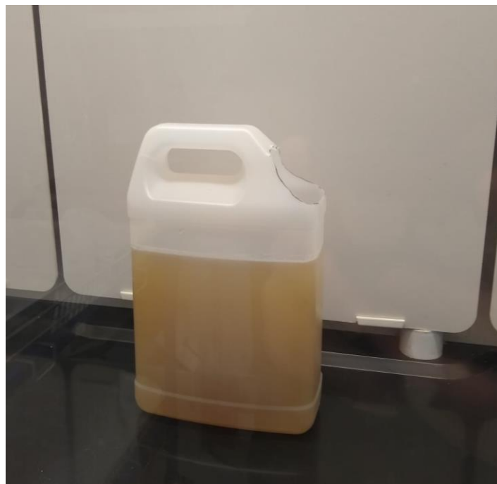
Figure S2-1. CBS-style container used in the experiment. The top was cut from a 1-gallon (3.78 L) container based on standard practices at SOIL.
