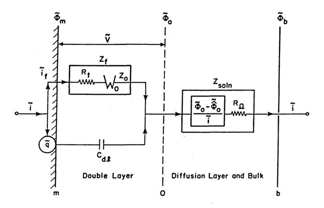
Figure 3. Schematic of the macroscopic model's breakdown of the electrochemical impedance.
