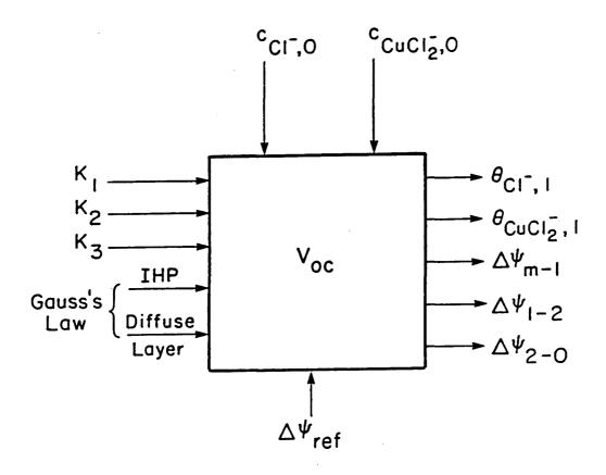
Figure 5. Schematic of the equilibrated-interfacial calculations made in the microscopic model.
