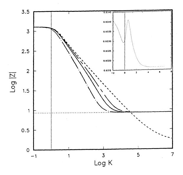
Figure 9. Bode plot of the total  $(C_{dl}=10~\mu{\rm F/cm^2})$ , faradaic, and solution impedances for copper dissolution. The S-M simulations are based on mechanism I and are denoted by solid, dashed and dotted lines, respectively. The total impedance based on  $C_{dl}=5$  and 30  $\mu{\rm F/cm^2}$  are given by chain-dashed and chain-dotted lines, respectively.
