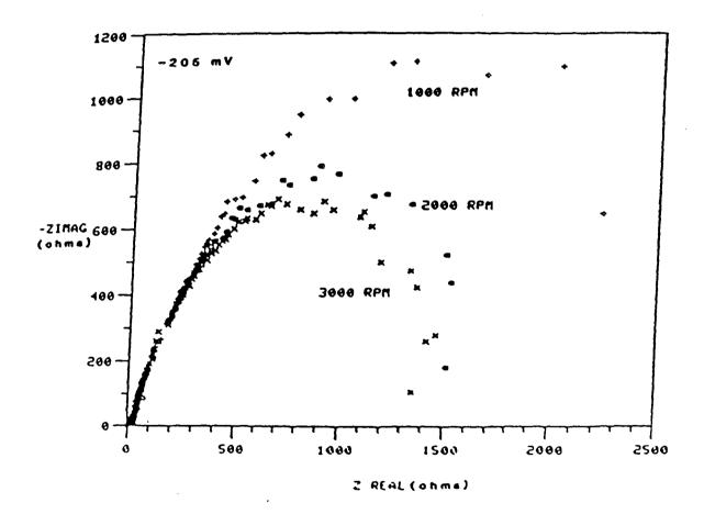
Figure 1. Experimental impedance data (from reference [4]) for copper dissolution in 0.1 N HCl as a function of rotation rate.
