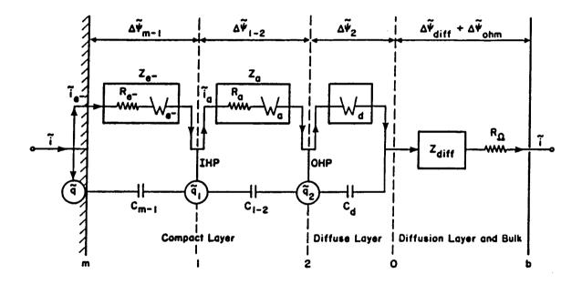
Figure 4. Schematic of the microscopic model's breakdown of the electrochemical impedance.
