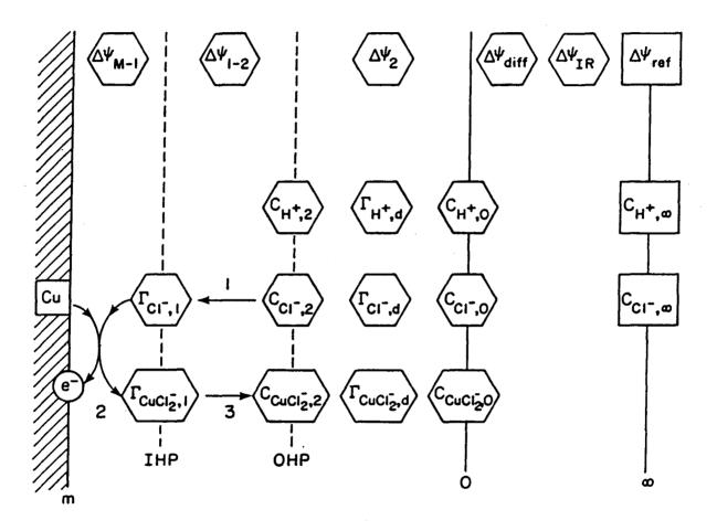
Figure 2. Variables in the microscopic model of the electrode-electrolyte interface when mechanism II is used.
