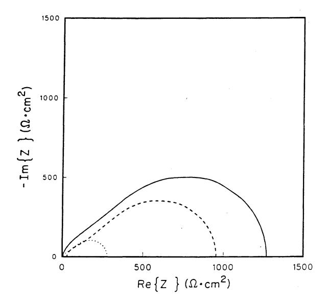
Figure 12. Complex-plane plot of the total, electron-transfer, and adsorption impedances as calculated by the microscopic model based on mechanism II (b) and denoted by solid, dashed, and dotted lines, respectively.
