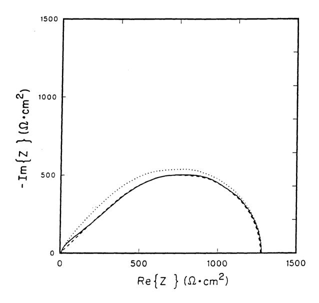
Figure 10. Complex-plane plot of the total impedance as calculated by the macroscopic and microscopic models based on mechanisms I (dotted line) and II (solid line), respectively. The Stefan-Maxwell faradaic impedance is denoted by a dashed line.
