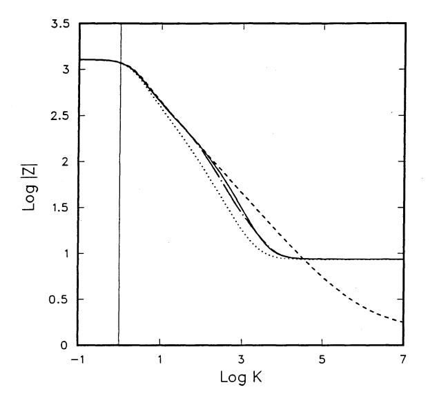
Figure 11. Bode plot of the total impedance as calculated by the microscopic model based on mechanisms II (a) and (b) and denoted by solid and chain-dotted lines, respectively. The Stefan-Maxwell total and faradaic impedances also are given and are denoted by dotted and dashed lines, respectively.
