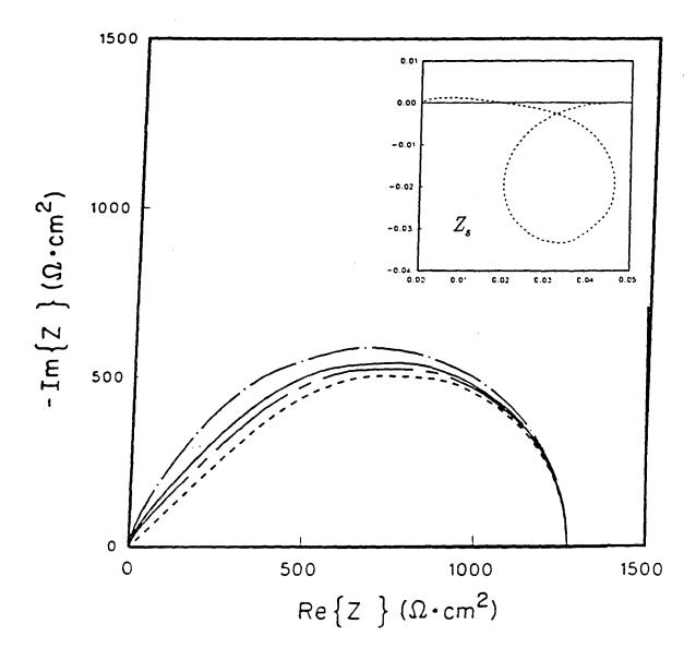
Figure 8. Complex-plane plot of the impedance for the anodic dissolution of copper as calculated by the Stefan-Maxwell macroscopic model based on mechanism I. Simulations of the total ( $C_{dl}=10~\mu F/cm^2$ ), faradaic, and solution impedances are denoted by solid, dashed and dotted lines, respectively. The total impedance based on  $C_{dl}=5$  and 30  $\mu F/cm^2$  also are given by chain-dashed and chain-dotted lines, respectively.
