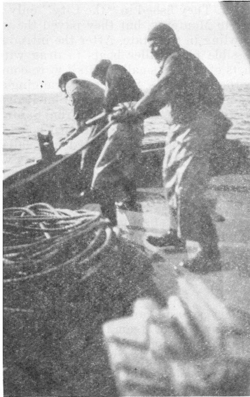
FIGURE 8. Paranzella trawling at Monterey, December 18, 1927. Warp being hand pulled and rope coiled on starboard after deck. Photograph by G. R. Chute
